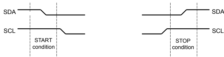
Figure 15-3. START and STOP Conditions
